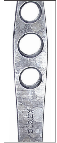
Spots caused by mineral deposits
